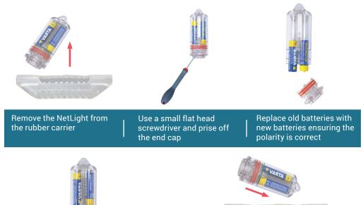
Click the endcap back onto the NetLight. Test the light is working Insert the NetLight back into the rubber carrier
